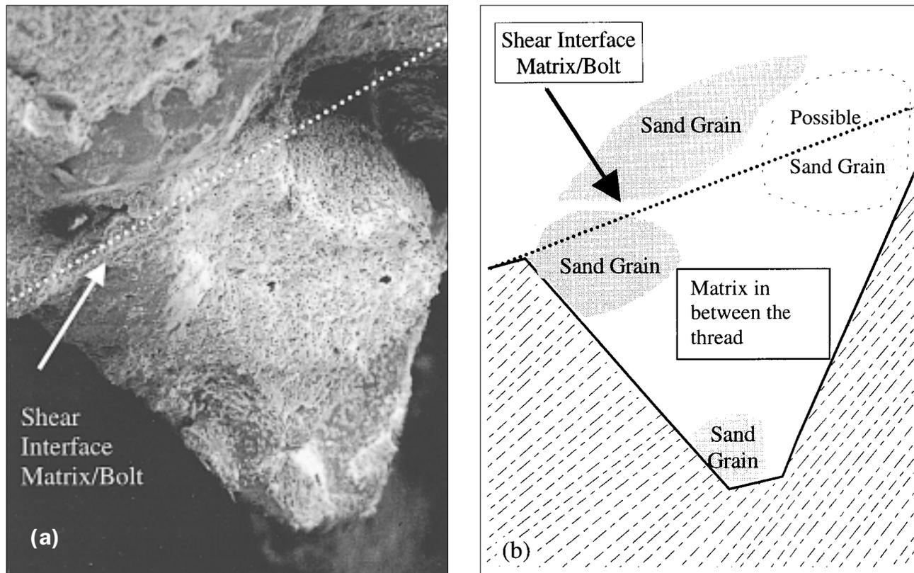
Fig. 8 – Dispersion of coarse aggregate in between and at the area of the threads: (a) SEM micrograph (100x), (b) sketch of the SEM picture.
