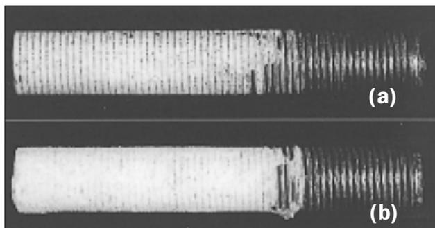
Fig. 7 – The threaded bolts after the pulling out from portland cement mortar: (a) coarse aggregate (374  $\mu\text{m}$ ), (b) fine aggregate (110  $\mu\text{m}$ ).
