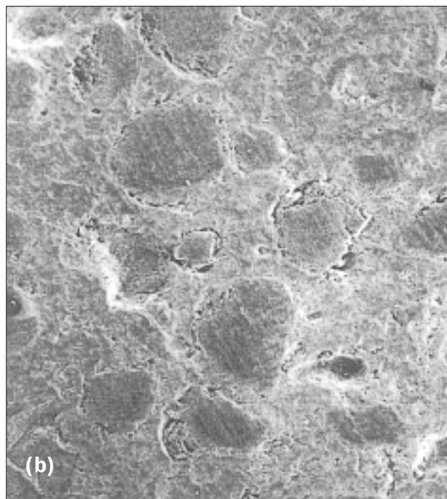
Fig. 3 – Microstructure of the two mortar systems (40x): (a) Wollastonite (b) Portland cement.
