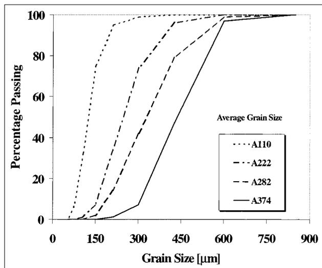
Fig. 1 – Sand grading curve and average grain size.
