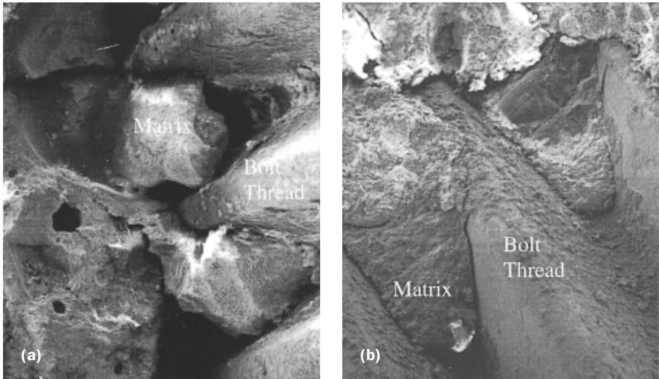
Fig. 12 – Penetration of the matrix in between the bolt threads (40X): (a) Wollastonite mortar, (b) Portland cement mortar.
