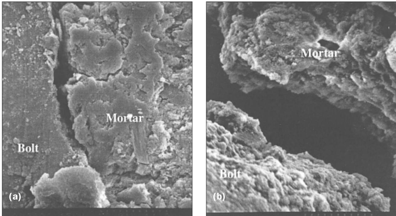
Fig. 4 – Bolt-mortar interface prior to pullout test x2000 (sand size 374  $\mu\text{m}$ ): (a) Wollastonite system, (b) Portland cement system.
