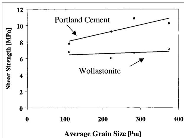
Fig. 5 – Effect of sand grain size on pull-out strength.
