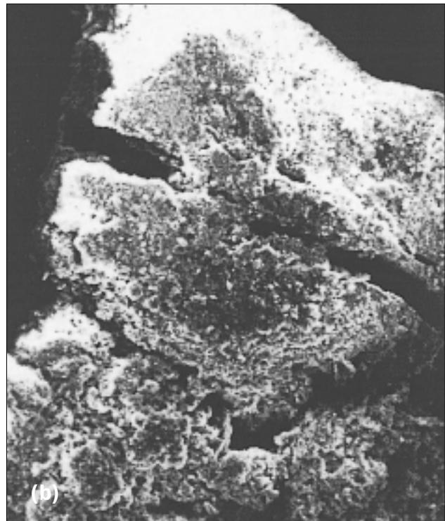
Fig. 10 – Coarse aggregate at the bolt-matrix interface after the pullout process, near the loaded end of the specimen: (a) uncrashed aggregate in Wollastonite mortar (110x), (b) crushed aggregate in Portland cement mortar (400x).
