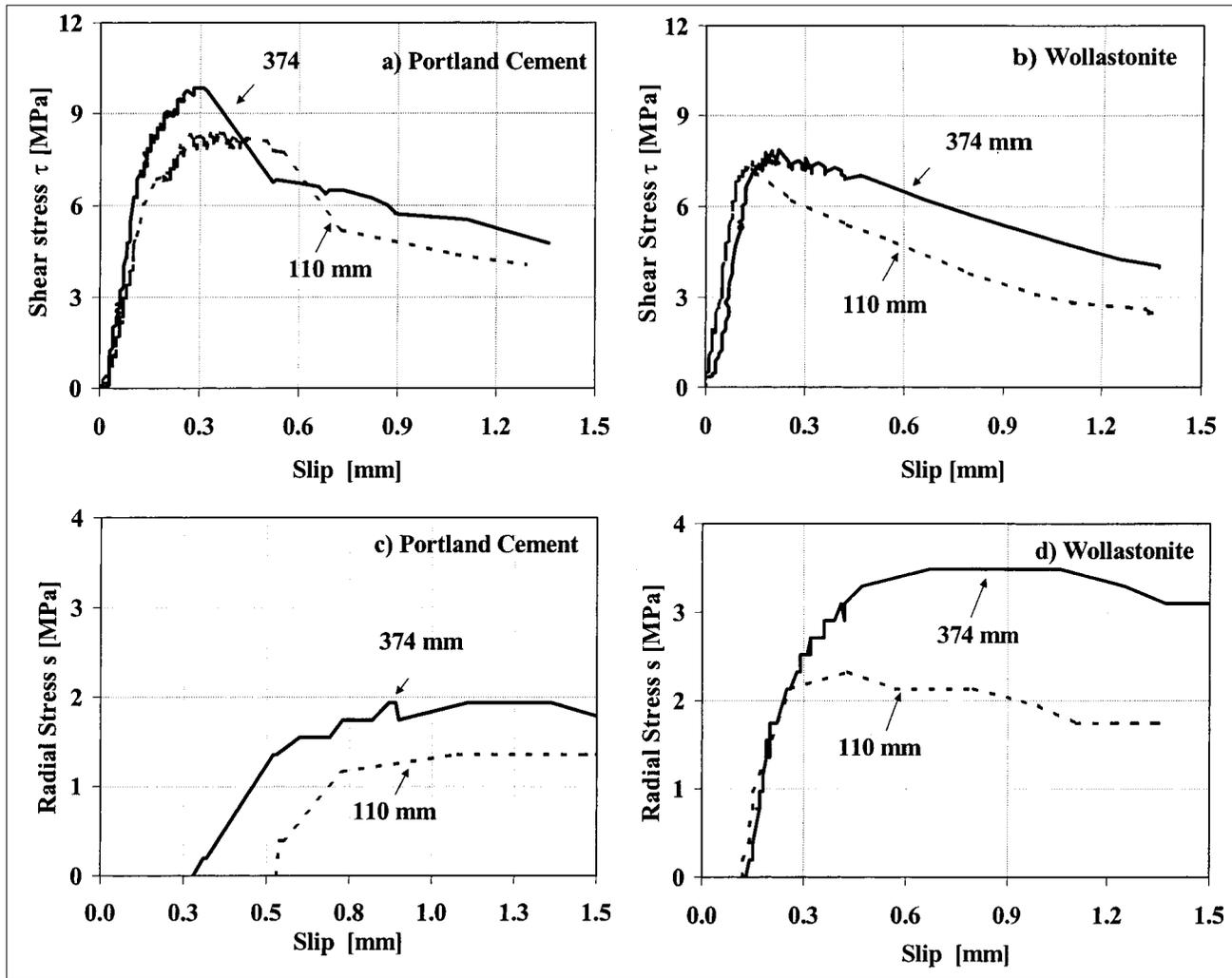
Fig. 6 – Shear and radial stress during bolt pull-out for portland cement and wollastonite systems: a) & b) shear stress vs. slip, c) & d) radial stress vs. slip.
