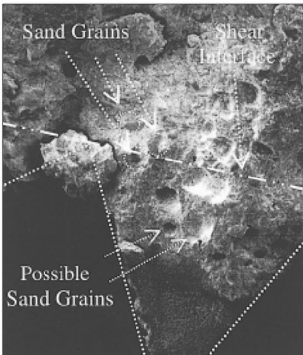
Fig. 11 – Dispersion of fine aggregates in between the bolt threads (70x).
