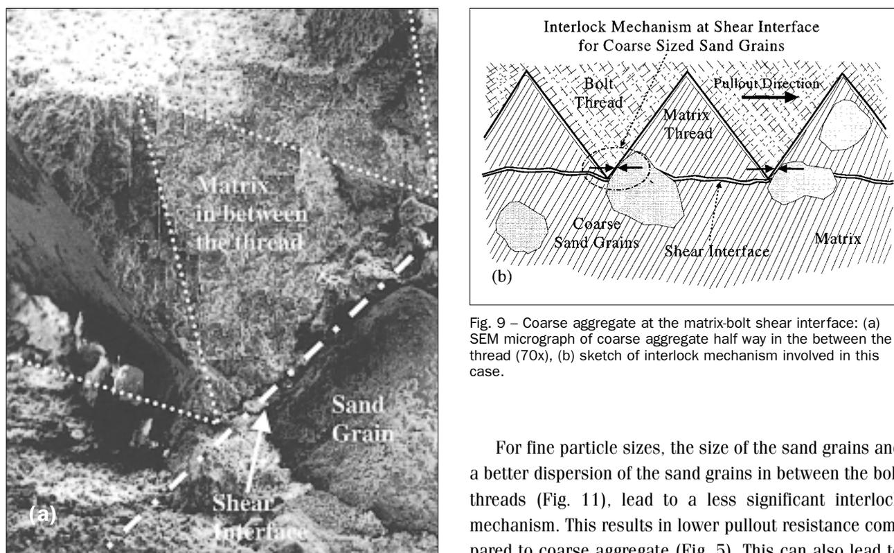
Fig. 9 – Coarse aggregate at the matrix-bolt shear interface: (a) SEM micrograph of coarse aggregate half way in the between the thread (70x), (b) sketch of interlock mechanism involved in this case.
