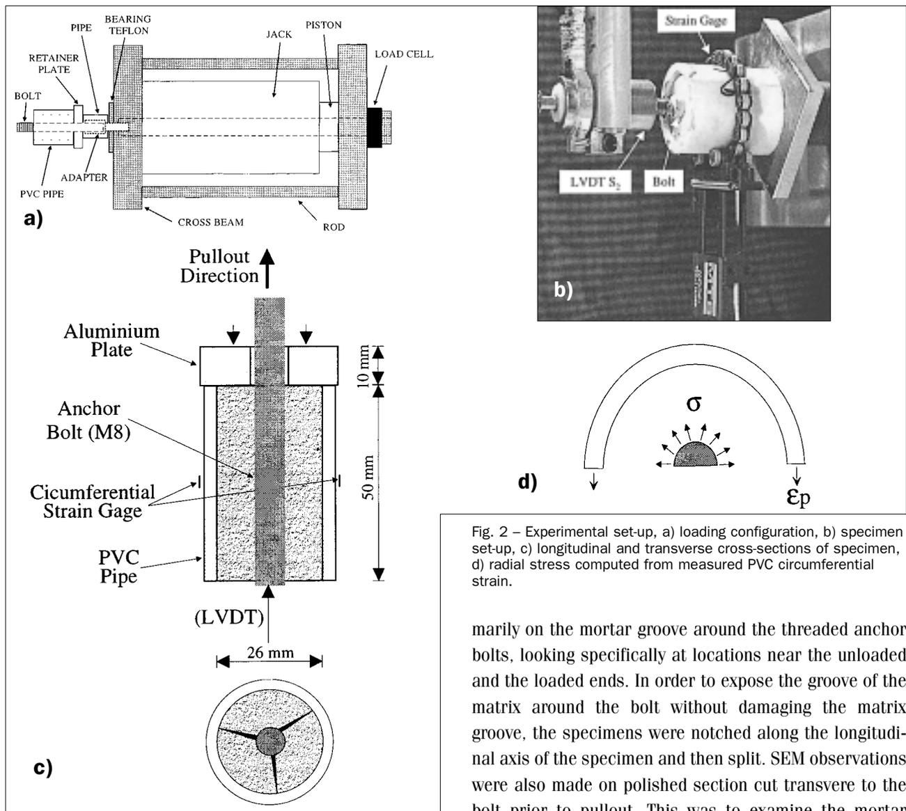
Fig. 2 – Experimental set-up, a) loading configuration, b) specimen set-up, c) longitudinal and transverse cross-sections of specimen, d) radial stress computed from measured PVC circumferential strain.
